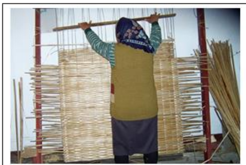
Photo 9. Weaving loom for mats
